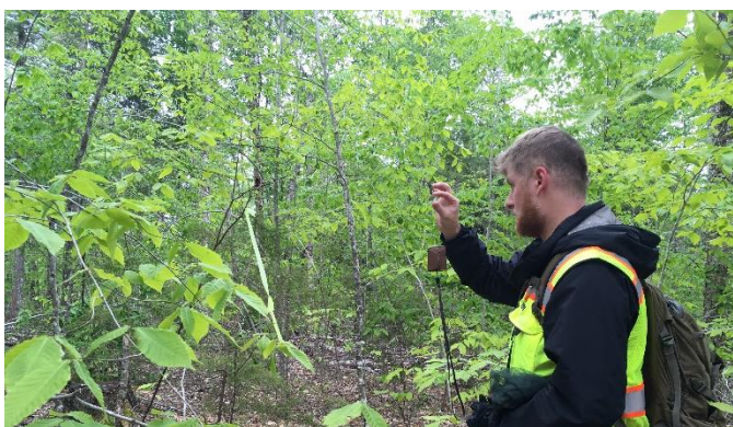
CFRU summer field crew member Jacob Burgess looks through a prism when conducting a variable radius plot inventory for the CFRU's Maine's Adaptive Silviculture Network. Researchers at the Wheatland Lab are evaluating the use of variable radius plots as calibration plots for LiDAR-based enhanced forest inventories. Image: J. Zukwert.
