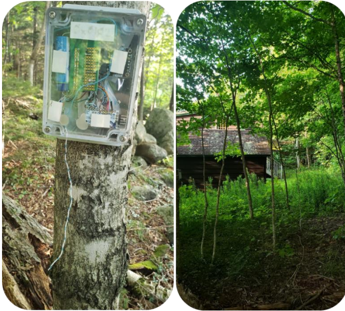
Figure 9. The deployment of wireless dendrometer and environmental sensors at INSPIRES partner, Appalachian Mountain Club's Pinkham Notch Visitor Center in New Hampshire, was successfully deployed in the fall of 2023. Photos provided by Dr. Jordon Tourville.
