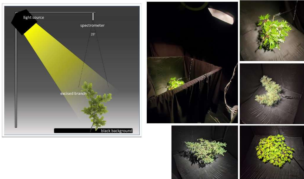
Figure 7. Diagram showing darkroom setup developed to measure the reflectance of individual branches (left). Photo of darkroom setup and examples of branches prior to measurement (right).
