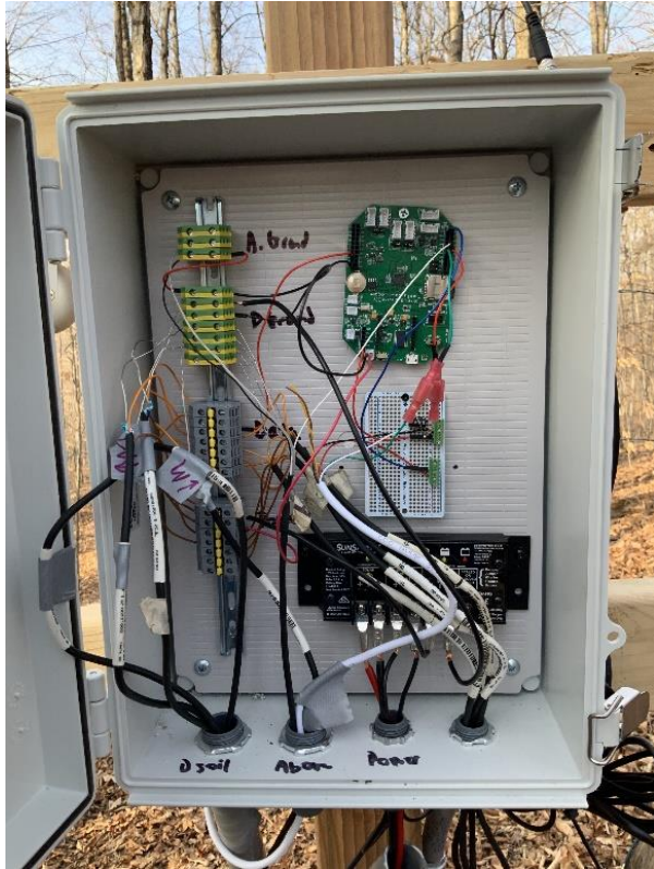
Figure 5. The “brain box” of the sensor suite houses the green Mayfly microprocessor, din rail and connectors, and black charge controller. The wires of all sensors feed into this box from the bottom ports to connect to power, receive and deliver data, and keep the system grounded.
