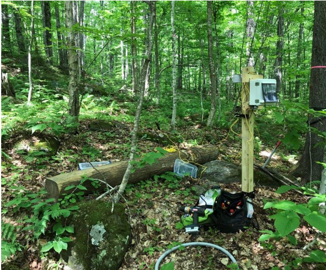
Photo 1. INSPIRES intensive sensor field site at Dartmouth Second College Grant Experimental Forest being used to monitor soil and wood moisture. (Photo courtesy Dave Lutz).
