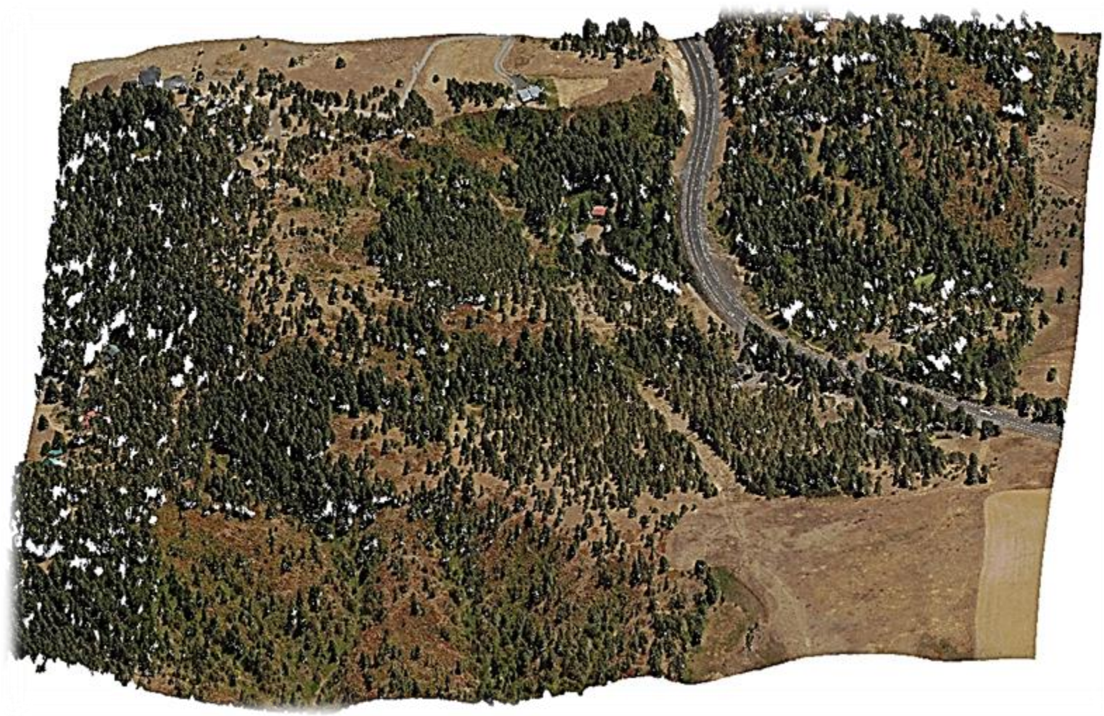
Colorized 3D NAIP Point Cloud (GSD: 30 cm, Frame Sensor)
