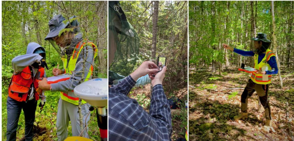
(LEFT): Casmir & Rissa recording data. (CENTER): Wayne calculating azimuth with a compass. (RIGHT): Casmir using a BAF prism to identify variable point samples.
