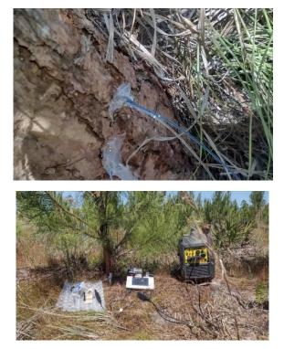
Long run time: 1-2 samples per day Sap flow changes with weather Probes break frequently
