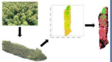
Drone captures high-resolution imagery of stands, image data passes through software to generate 3-dimentiounal point clouds and canopy height models, clustering algorithm used to create stratified plots.
