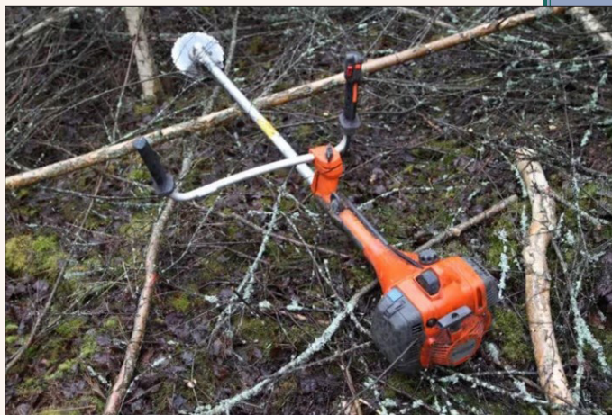
Figure 3.4 . Scandinavian spacing saw widely used for precommercial thinning.
