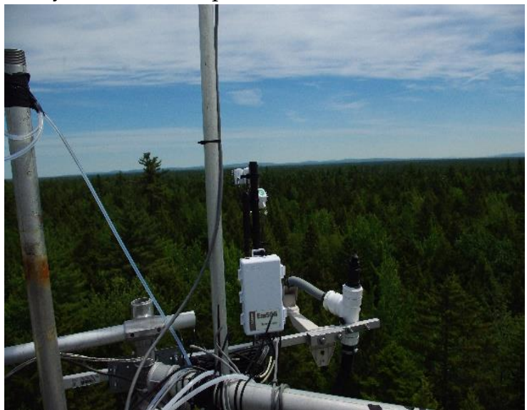
Instruments collect flux data at the top of the main Howland Research tower. Photo courtesy Meg Fergusson.
