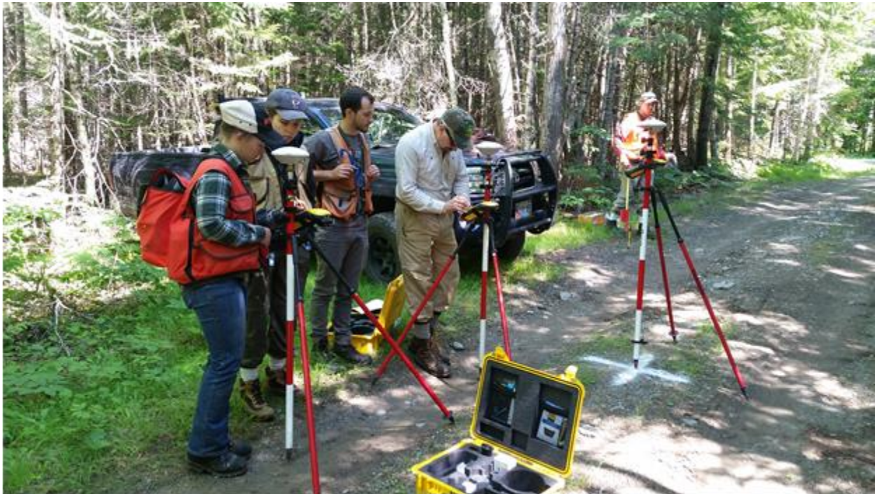
From left, Lauren Keefe, Jamie Behan, Jim Alt, Tony Guay, and David Sandilands from University of Maine setting up three Trimble Geo7x's for ground control point (GCP). Photo courtesy Bethany Muñoz.
