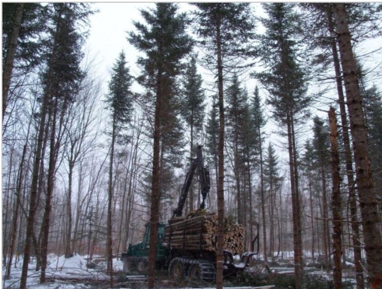
Forwarder collecting wood in a timed trial at the Austin Pond Study (Patrick Heisl photo).
