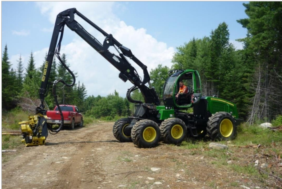
A John Deere 1170E Cut to Length harvester at the Early Commercial Thinning Study site in Summit Township, Maine (Jeff Benjamin photo).
