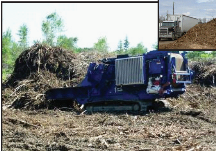
Modern grinder in the woods for grinding biomass.
